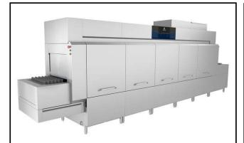
520122 (EFTD082EL2U2D1M5ER386) Flight Type Dishwasher, 3 tanks, 8200 dishes/h, electric, 950mm loading, 1300mm unloading, 1 dryer, 55mm conveyor, ESD, right to left
